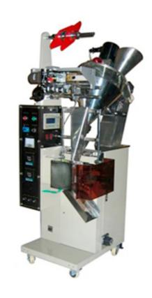
This packing machine is for granule, powder, nut, in chemical industry, pharmacy and food stuff industry.
