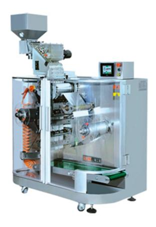
The NSL260 is a high-speed Strip Packing Machine and has been designed to pack capsules, tablets, or similar products.
