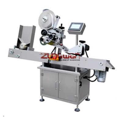
It is used for automatic labeling and printing different bottles in pharmacy industry such as ampoule bottle, vial bottle, oral bottle and so on.
