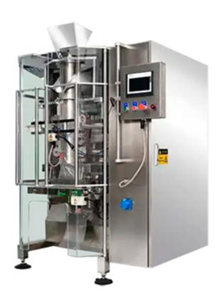
BVL-420 is specially designed for back-sealing bags and pin-back sealing bags. It is suitable for smaller back-sealing bags. The bag width it can make is 80-200mm and the bag length is 80-300mm. The fastest can reach 80 bag/min. It can package salt, chicken essence, white sugar and other granules, as well as water, oil and other liquids, and has a wide range of applications.
