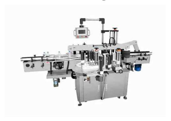
Feeding  $\rightarrow$  bottle dividing  $\rightarrow$  synchronous pressing  $\rightarrow$  labeling  $\rightarrow$  pressing label  $\rightarrow$  online inspection and rejection  $\rightarrow$  finished product.
