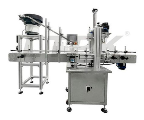
This LTPK LT-CZJ60A Automatic capping machine with vibratory cap feeder is equipped with a cap feeder, which can orient bottle caps. Typically the cap feeder can be customized by making adjustments to the bowl for different sizes of caps. Larger caps and higher speeds may require larger bowls.
