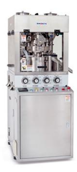
Tablet Press – PILOT 200 DL is a High Tech Double Layer & Monolayer Rotary Tablet Press is essential for R & D and small batch production. This Single sided R & D Double Layer Tablet Press fully conforms to GMP and the safety requirements, featuring versatility with a quick change of tooling.
