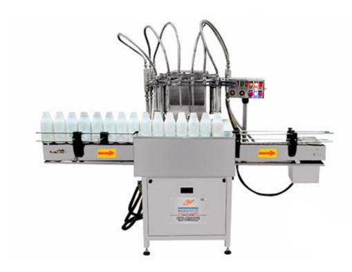
The Automatic Volumetric Liquid Filling Machine consists of a main structure, product transmission belt with an adjustable guide, safety acrylic enclosure with SS pipe frame (OPTIONAL), pneumatic/mechanical stopping facility, nozzle & syringes, electrical panel, motor, sensor, AC drive & mains ON/OFF.
