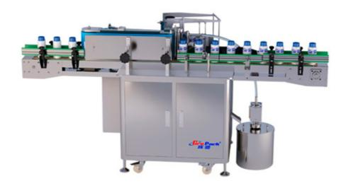
The labeling machine is used for a round bottle with cold glue applied. It is largely applied in the food industry.
