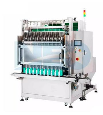
The bottle unscrambler BU5500 is easy to operate, understand and maintain. When using, operator only need to put the bottle container into the empty bottle storage tank. Bottle elevator will then feed the bottle to the bottle unscrambler. The bottle unscrambler system will automatically organize all bottle into order with orderliness orientation.
