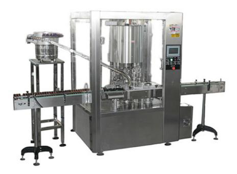
This machine is used to seal all kinds of tinplate cans, aluminum alloy cans, paper cans and other round specification cans, easy to operate and learn.
