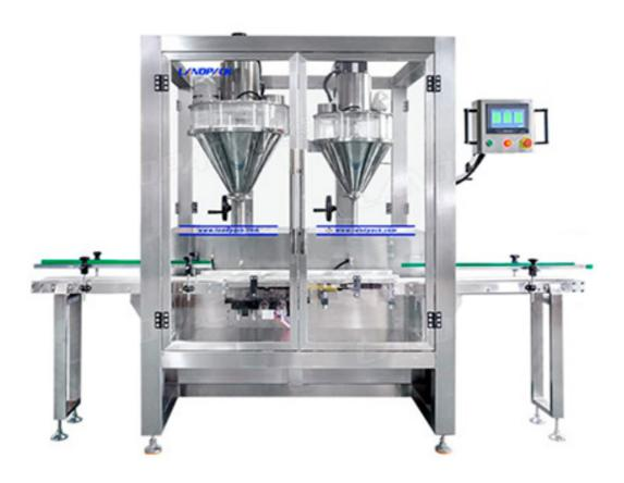
Double heads automatic powder filling machine is suitable for all kinds of powdered, ultrafine powdered or powder granular material, canned, bottled, barreled. Such as: talcum powder, rice flour, protein powder, cocoa powder, coffee powder, powdered drugs, chicken powder, chicken, additives, sugar, dyes, flavors and spices, etc.
