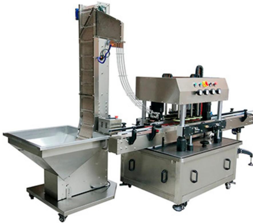
Automatic 8-Wheel Spindle Capping Machine with an Automatic Cap Feeder is designed for high-speed, reliable, and consistent capping of bottles and containers with screw caps. This machine is commonly used in industries such as pharmaceuticals, cosmetics, food, and chemicals, where efficiency and precision in capping are crucial.
