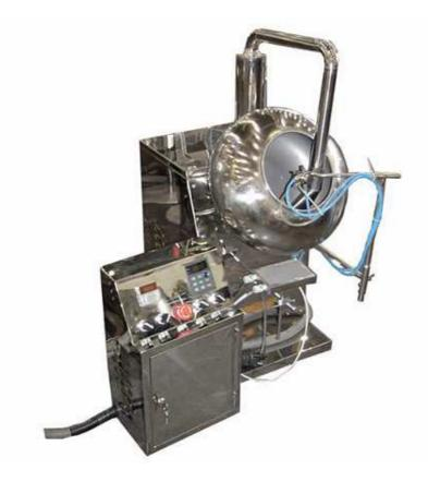
The machine is used to carry out sugar coating and so on to the core of Chinese traditional medicine and western medicine tablets, it integrates strong power, weak power and hydraulic pressure with pneumatic operation, it is new type equipment improved on the basis of original common type sugar coating machine.
