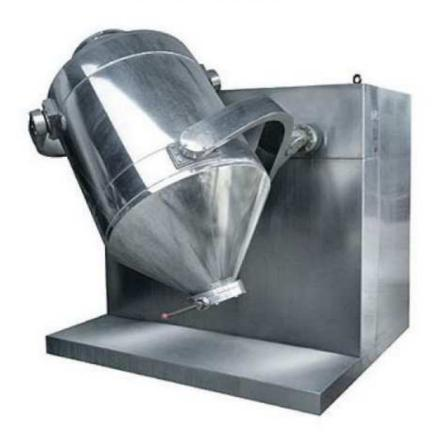
This new designed mixer is widely applied in pharmaceuticals foodstuffs, chemical, industries and light industries to mix dry powder and granulator.
