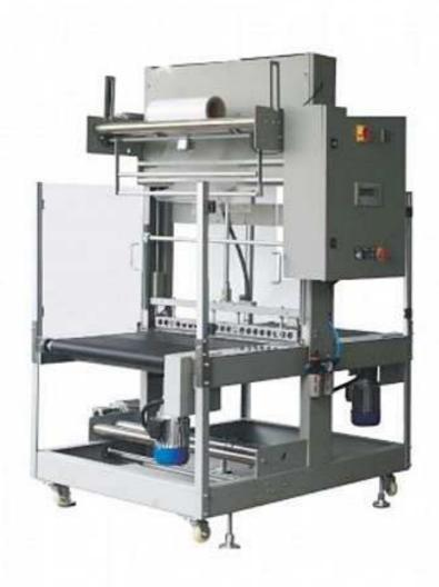
Shrink wrap machines apply heat to shrink a plastic film around a product. This process is often done by automated equipment, but manual and semi-automatic shrink wrap machines are also available. Shrink wrap machines cover the item, and then sent it through a heat tunnel or oven for shrinking.
