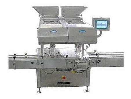
SL-A Series Electronic Tablet/Capsule Counter is specialized for counting the products of medicine, health care, food, agricultural chemicals, chemical engineering and so on. For example: tablets, coated tablets, soft/hard capsules. The machine can be used alone as well as with other machines produced by our company to form a complete producing line.
