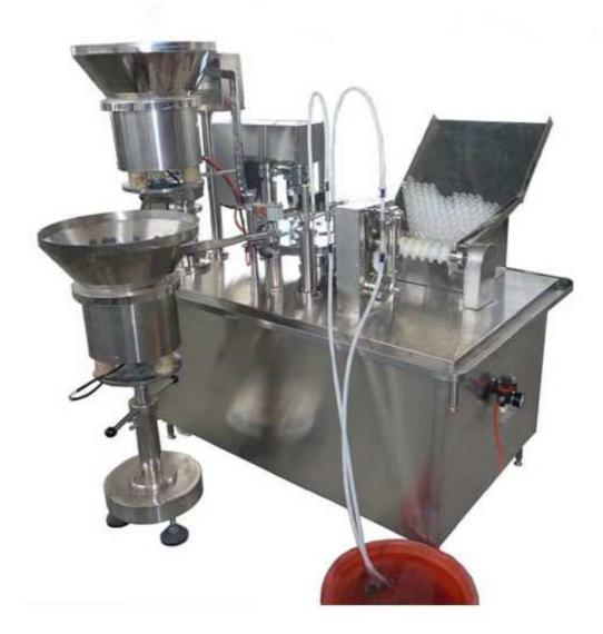
This machine is the main filling equipment of the sanitarian or syrup assembly line, which is mainly applied in the filling, lading and revolve, sealing of the 50-200ml plastic bottle transportation by feed bottle cover, track the local filling process, and is not easy to produce foam; it transports the lid by electromagnetic vibration with high lading rate. This machine is advanced in its combined filling-sealing operation with the compact structure.
