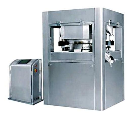
Multisession high speed tablet press GZK730 / GZL430 for pressing granular materials into round tablet form. It has high performance; it can be seen from the table below. The molding process also participates accessories (servo motor, modular roller device), which helps to work efficiently and powerfully, and therefore is used in the modern pharmaceutical industry and for the manufacture of tools for the health care.
