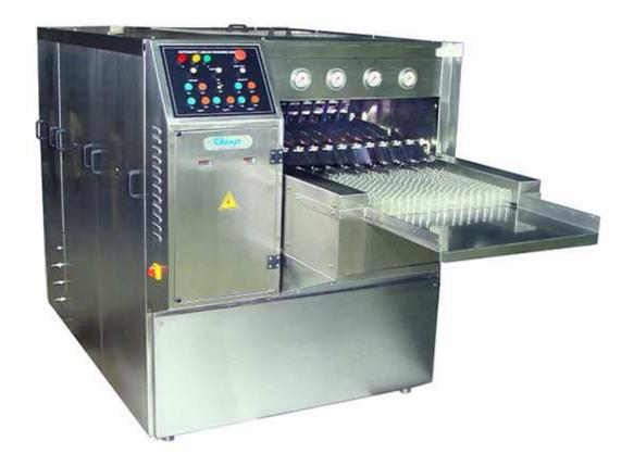
High Speed Linear Vial Washing Machine is most ideal for Round Vial and finds wide application in PHARMACEUTICALS INDUSTRIES. The automatic loading arrangement facilities loading of vials on to SS wire mesh conveyor through feed conveyor or vials are pushed manually from feed table. This saves manpower as vials are feed into pockets automatically. The automatic unloading mechanism consists of unloading vial continues on to turn table (Optional).
