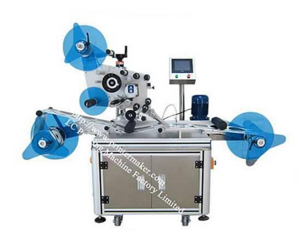
This machine is used for Rolling Labeling
