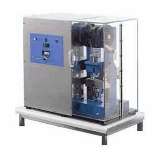
TP1400 tablet compression machine is made of stainless steel and easy to operate. The tablet diameter and size can be adjusted by replacing the base formation or displacer. Two steel cams control stepping, does not need to adjust. The raw materials are placed in a vibrating vessel which is shoes shape, when the quantity is big; an external connection hopper is optional. The finished products discharge from a skewed slot, a collecting vessel can be placed here.
