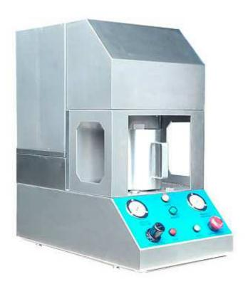
In the relatively airtight environment-working cabin, use high and low pressures to alternate changes rapidly "pressure shear" causing pulsed drawing force to the capsule. Under the continuous function of the pulsed drawing force, the capsule is gradually drawn and separated.
