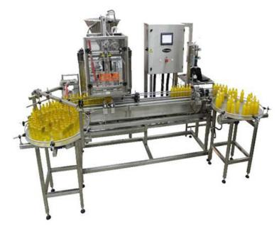
The SILVER filling and capping machine meets most requirements of filling liquid products, in different viscosity levels, such as: syrup, oil, sauce, ketchup and more.
