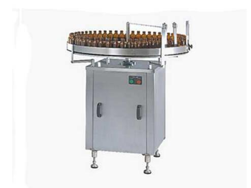
Turntable is useful to ensure total synchronization, uniform flow of container and to take a turn at 90 degree to suit different machine and purpose in automatic liquid line.
