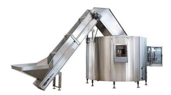
LPJ serial full-automatic bottle unscramble is the support equipment for the soft beverage filling equipment, applicable for the orderly arrangement of messy PET bottles and the delivery of them to production line.
