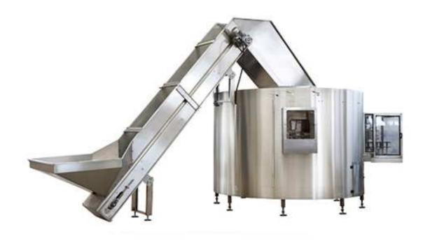
The machine is used for ordering disordered polyester bottles. The disordered bottles are carried into the storing bottle section by elevator. With the help of the pushing force of the rotating disk, the bottles enter their position. With the function of the turning bottle device and the air-flow, the bottles are ordered into bottle mouth-up-position and are carried into the next process with the air-transferring type conveying bottle system.
