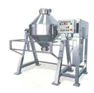
We are a noteworthy supplier of Double Cone Blender for our huge clientele base. It is used to mix granules and dry powder homogeneously. Contact parts of this blender is made out of stainless steel along with the help of advanced machinery at our unit. Double Cone Blender is known for being user- friendly, durable, efficient, effective, durable, highly functional and its long operational life. This has gained us high rising demands for this blender among that of our competitors.
