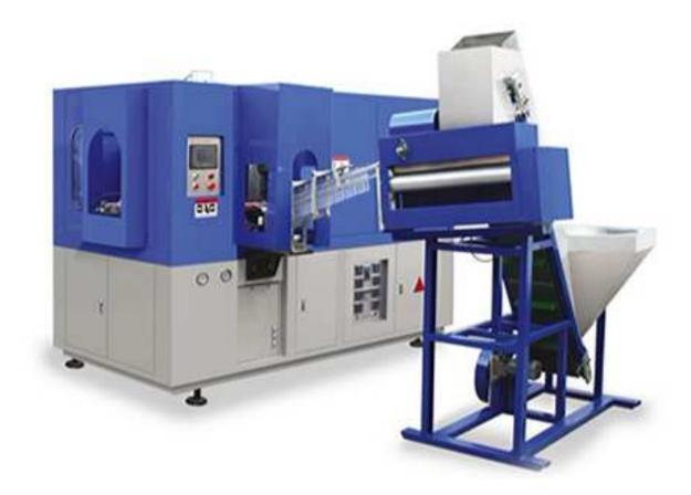
Full automatic blow molding machine is suitable for producing PET plastic containers and bottles in all shapes. It is widely used for producing the carbonated bottle, mineral water bottle, pesticide bottle, oil bottle, cosmetics bottle, wide-mouth bottle and hot filling bottle etc.
