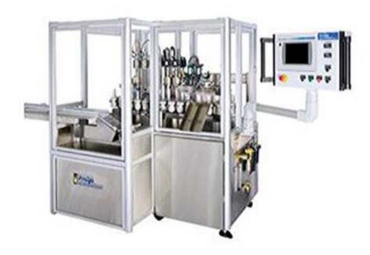
The PROTRAC system with speeds to 220 airless pumps per minute features a race track design, dual filling and closing stations as well as multiple post filling options.
