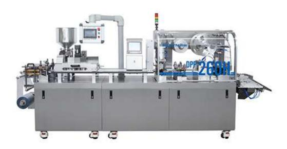
The machine integrates light, machinery, electricity and gas, which is controlled by PLC programmable. Which can automatically completed the process of forming, feeding, heat sealing, creasing and cutting. Applicable to pharmaceutical, food, electronics, medical equipment, hardware and other industries of aluminum-pvc, paper-aluminum, aluminum-aluminum and other packaging.
