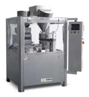
NJP series fully automatic capsule filling machine are newly invented machine, which is produced to meet high production capacity requirement on the basis on original NJP series capsule filling machine. These two machines have dual capsule turn around device, and dual capsule whole moulds. It can increase the production capacity without increase operator and space.
