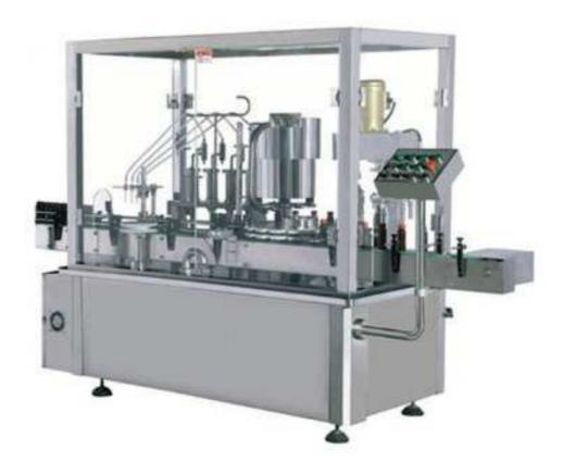
SED-4/1GX Automatic Filling and Capping machine for the application of light liquid filling and capping for plastic or glass bottles. The machine is composed by a conveyor, SS316L volumetric piston pump, top-bottom filling nozzles, liquid buffer tank, bottle index wheel, capping system. The bottle loading/unloading through loading/unloading turntable (alternative Ø620mm or Ø900mm), or directly from an production line.
