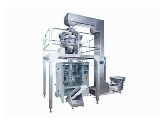
VFFS machine has a wide range of application for industries. It's greatly meet the factory's needs for production. Especially, food and fast consuming products that need a lot for vertical form fill seal machines. Variable package types, fast packaging is the main factor for the needs. VFFS 520 has a middle pouch size application whose max. width is 245mm. The speed can be up to 70 bags per minute.
