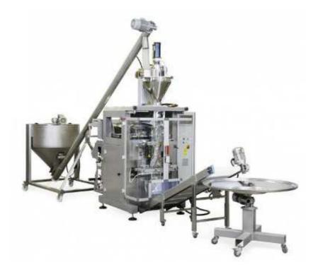
This is a fully automatic vertical form fill seal bagger, which is applicable for packing different products with correct filling system. Such as coffee capsules, coffee powder, coffee beans, chocolate cream, pet food etc. This machine is very popular used in food, chemicals, construction, tobacco, fertilizer, medical, pharmaceutical area.
