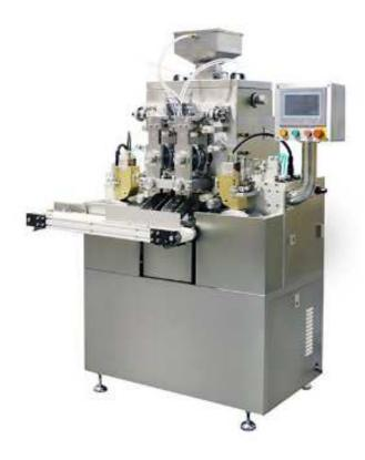
This is small experimental equipment, suitable for new product experiments, which can then be reviewed before use. It is compact in structure, with a patented pendulum align die roll and an open housing assemble structure, easy to use and maintain.
