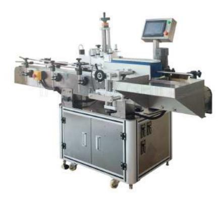
Vertical type Automatic Labeling Machine. It adopt vertical type transmission, vertical type labeling, more stable, more precise and improve working efficiency.
