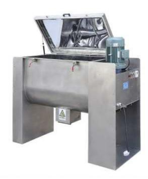
Ribbon Blenders consist of a U-shaped horizontal trough, transmission parts and ribbon agitating blades which usually have double or triple layers with outside screw gathering the material from sides to center and inside screw transmitting the material from center to sides to form convection mix and a specially fabricated ribbon agitator.
