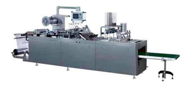
This blister packing machine which is suitable for "PVC/PET blister + Card" packaging for such as battery, glue, lipstick, pen, injection, toy gun, buring torch, toy car, scissor, alarm, toothbrush, coat & hat hooks, chopsticks, cleaning balls, bottle openers and so on.
