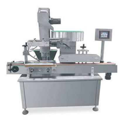
High speed pressure capping machine adopts rotating disc to arrange caps, low noise and stable cap conveying, Caps can automatically full back into cap hopper if they are in wrong direction, ensure the accuracy of capping.
