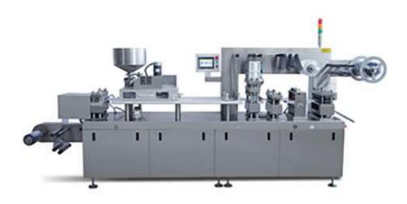
The contact part of the drug is made by stainless steel and high grade aluminum alloy materials, It is fully abided with GMP requirement. applicable to the pharmaceutical, food, health care products packaging industry plain tablets, sugar coated tablets, capsules, can be packaged honey pill, cosmetic, injection and so on. Aipak® is best tablet blister packing machine manufacturers. Alu Alu blister packing machine.
