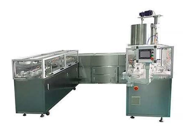
SP- 7L type full automatic filling production line has a stable and efficient suppositories preheating mold, heated mold, molding, belting, canned, frozen, sealing bolt all production processes such as complete system process, grain production capacity of 8000-12000 / hour.
