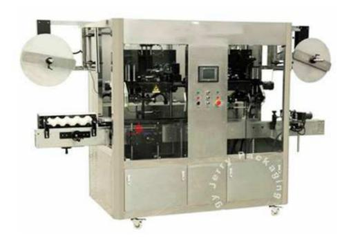
The machine is designed to label bottles with sleeve labels made of PVC, PET, OPS and other heat sealable films. Film thickness must be within 0.03-0.13 mm. Applicable bottles must be within 25-14 mm in diameter, made of glass, metal or plastic and must be square, flat, curved or cup-shaped.
