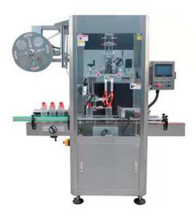
HF-250M is single head and single driving machine, the max speed 250bottles per minute (by sleeve height 5~10cm) are common used, meet most user's requirement.
