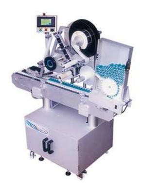
Wrap-around labeling of tubular bottles (that cannot stand upright) on the round barrel portion; can be added with an automatic star disc feeder.
