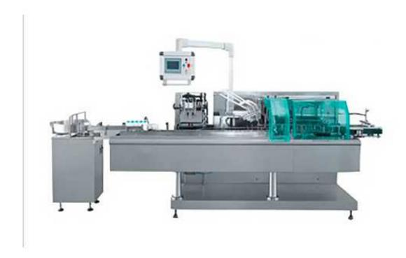
Cartoning machine is a kind of packaging machinery, including automatic cartoning machine, medicinal cartoning machine and so on. The automatic cartoning machine automatically loads the medicine bottles, medicinal plates, ointments, etc. and instructions into the folding carton, and completes the box closing action. Some of the more functional automatic cartoning machines also have sealing labels or heat shrink wrap. Package and other additional functions.
