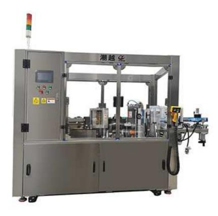
This labeling machine is a new concept in labeling. It uses continuous operation to cut the labels, apply glue and then paste them on the container, instead of cutting or stacking the labels in advance.
