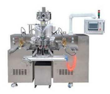
KY-250 soft capsulation production line is of large scale production equipment. The single unit annual production capacity is 4 hundred million capsules. Adopts international advanced control technology, precisely design precisely producing, it is the dependable equipment for the production of high quality soft capsules. Humanized design, easy to operate .The mold matches the mold shaft, to avoid damage in the process of loading and unloading.
