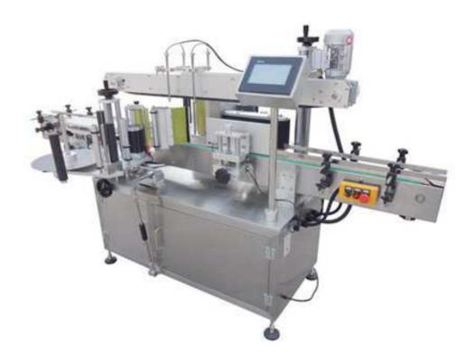
The TS-150B multi-function double-sided marking machine consists of the pressure marking mechanism, bidding head, frame mechanism, bottle separation unit, bottle transmission mechanism, adjustment mechanism and electrical box. The machine has mature technology, high marking accuracy, stable and reliable action for flat, square and round bottles.
