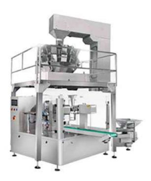
This set of equipment is mainly suitable for automatic counting and packaging of small bags (like medicines, coffee, cereal, cold granules, etc.). After lifting the pouch material into the automatic metering device by the hoist, the computer automatically combines the set quantity, and automatically packs, seals, and outputs the finished product by the bag type packaging machine, and the whole set of equipment is highly automated.
